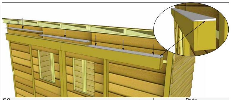
**56.** Position **4KD - Track Overlay - Sill** pieces evenly on top of Track Overlay with the slope facing away from the shed. This will prevent rainwater from collecting on top. Attach with **3 - 1 1/2" Finishing Nails** per piece. Hammer carefully and support the Track Overlay from below if necessary to avoid knocking it loose.
