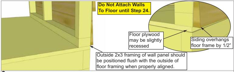
**9.** The side wall panels will sit even with the floor frame and the rear panels will be sandwiched between the side wall panels. The floor plywood may be slightly recessed. **Note:** Siding will overhang the floor frame by approximately 1/2".
