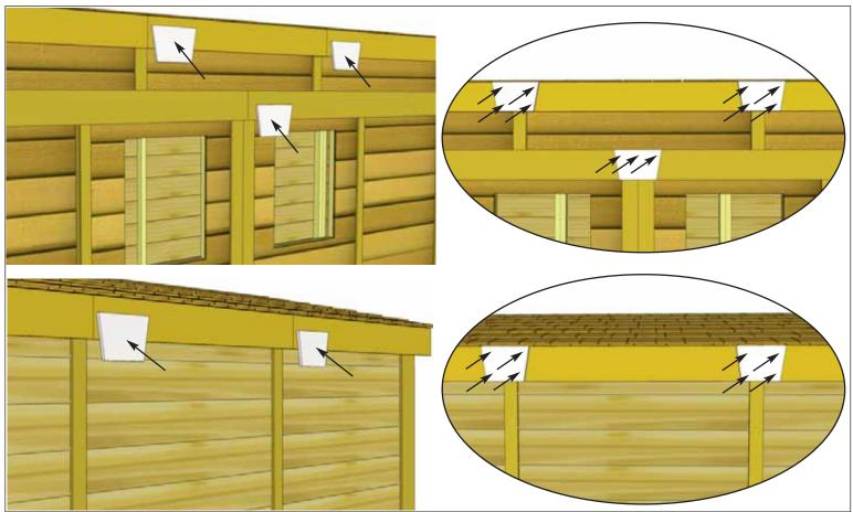
**65.** Attach **4U - Trim Detail Plates** to cover seams. Four Plates will cover seams where Front and Rear Facia pieces meet, attach these with **4 - 1 1/2" Finishing Nails** per piece. One more Trim Plate will cover the seam of the Track Overlay, attach with **3 - 1 1/2" Finishing Nails** along the top of the Plate so nails are secured to 2x4 backing.
