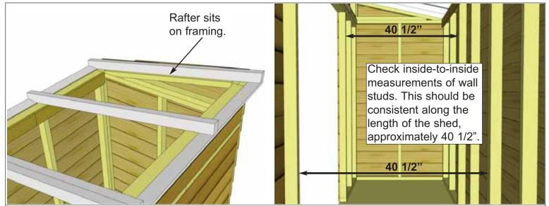
**27.** Position completed Rafter Section on top of walls. Outside Rafters will sit on Extension Wall framing and be positioned equally from side to side.
