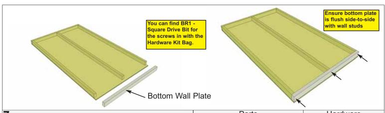
7. Carefully lay 2AA - Side/Rear Wall Panels face down. Position and attach 2AB - Bottom Wall Plates to bottom of wall studs of each wall panel with 3 - 2 1/2" Screws. Position so plates are flush with framing. Complete 4 remaining solid walls.
