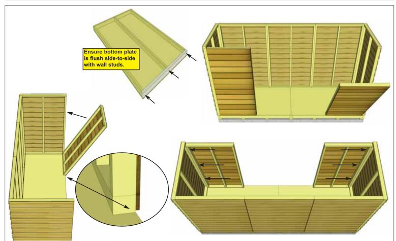
13. Carefully lay 2BA - Front Wall Panels face down. Position and attach 2BB - Bottom Wall Plates to bottom of wall stude of each wall panel with 3 - 2 1/2" Screws as per Step 7. Complete other remaining Front Wall.
