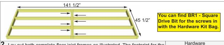
**2.** Lay out both complete floor joist frames as illustrated. The footprint for the floor when attached together will be 141 1/2" wide x 45 1/2" deep. Attach frames together with **6 - 2 1/2" Screws.**
