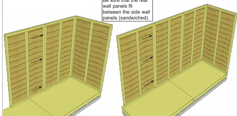
**11.** With the corner wall attachment complete, position a second rear wall panel in place so bottom 2x3 wall framing is sitting flush with outside floor joists. Wall siding should overhang floor by approximately 1/2". When positioned correctly, attach both side wall panel study together as per **Step 10**.
