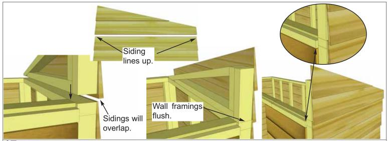
**17.** Align wall framing of Angled Wall Extender and Side Wall so they are flush at the front. The siding for both walls should also align evenly from front to back.
