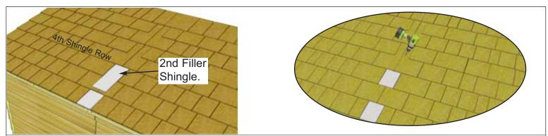
**39.** Slide 2nd **Filler Shingle** up and underneath fourth shingle row. Follow **Steps 37 - 38** to align and attach. Repeat for other roof seam.
