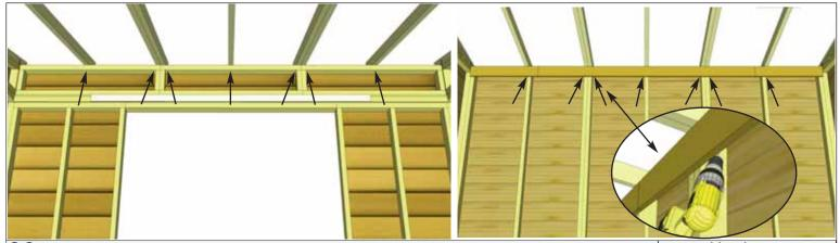
**30.** With outside rafters properly secured, attach remaining interior rafters using **1 - 3" Screw** per rafter end. Screw into rafters from inside of Wall Extender framing at front of shed, and from inside of Rear Wall top framing at rear of shed, behind Horizontal Wall Cleats.
