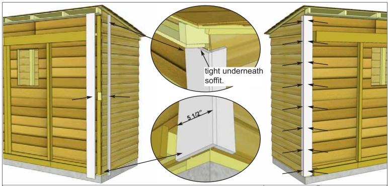
**57.** Place **4L & 4M - Front Corner Trims** in front corner and align as illustrated above. Do a dry run prior to attaching to achieve best fit. Start with 5 1/2" wide Front Corner Trim and align tight underneath soffit to determine vertical height. Attach with **8 - 1 1/2" Finishing Nails** per piece. Position and attach Side Front Corner Trim (2 1/2" wide) using **8 - 1 1/2" Finishing Nails**, aligning at bottom with wide trim.
