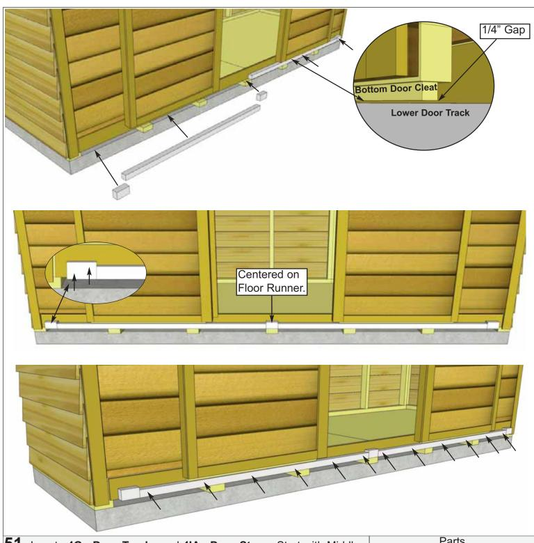
**51.** Locate **4G - Door Tracks** and **4IA - Door Stops**. Start with Middle Door Stop centered on middle Floor Runner and build out from there. Door Tracks rest on Long Floor Runners. Bottom of Door Stops and Door Tracks should be flush with each other. Secure Door Tracks to shed with **6 - 3" screws** per piece. Secure Door Stops with **2 - 3" screws** per piece.
