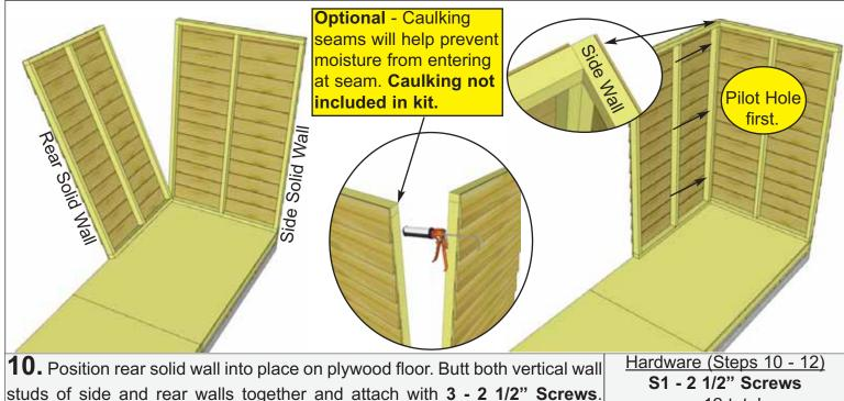
Screw at the bottom, middle and top of stud to secure properly.
