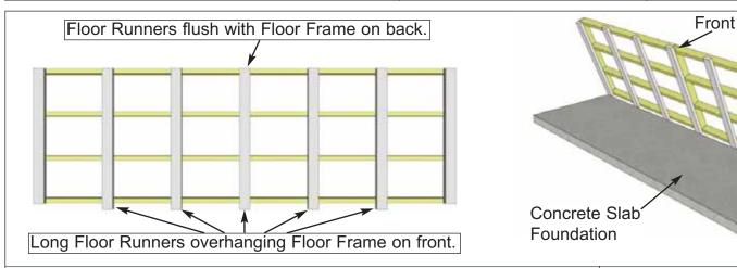
4. Align 1CC - Floor Runners - Long evenly spaced as shown above and flush with the back of the Floor Frame. On the front, Runners will extend 2" past the Floor Frame to provide support for the Sliding Door Track later in the Assembly. Attach with 4 - 2 1/2" Screws per Runner. With Floor Runners attached, carefully flip the floor over and place on your
