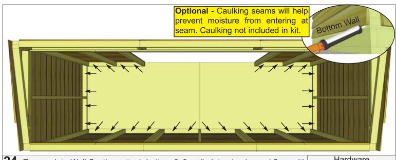
**24.** To complete Wall Section, attach bottom 2x3 wall plates to plywood floor with **2 - 2 1/2" Screws** per wall section. Prior to securing, make sure wall panels are aligned correctly on the floor. Refer to **Step 9.** Wall siding should overhang floor while 2x3 wall plates should sit flush with floor.
