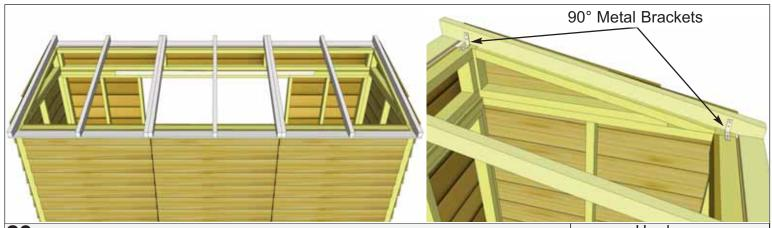
**29.** With Rafter Section correctly aligned, secure rafters to walls using **2 - 90° Metal Brackets** per side. Attach each brackets with **4 - 1 1/4" Screws**. Screw into Wall Extender framing at the front and Wall Panel top framing at the rear. Complete both sides.
