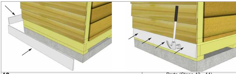
**43.** Attach **4A - Side/Rear Bottom Skirting** around the base of the shed. Skirting will hide floor framing. Start with side skirting pieces first and attach with **4 - 1 1/2**" **Finishing Nails** per piece.
