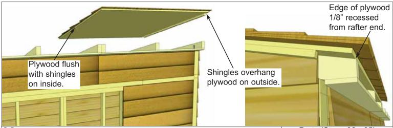
**32.** Correctly orientate **3G - Side Roof Panel**, with shingles overhanging plywood on the side of the shed and flush with plywood toward the center of the shed. Place on rafters with rear edge of plywood just about flush with rafter ends but just slightly recessed. Doing so allows rear facia to sit better.
