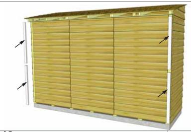
**48.** Position and attach **4D - Rear Corner** Filler Trim with 4 - 1 1/2" Finishing Nails per piece as per Step 47.
