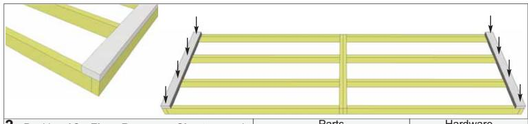
3. Position 1C - Floor Runners - Short on each side of the completed floor frame. Runners should be flush with corners but not overhanging. Attach with 4 - 2 1/2" Screws per Runner.
