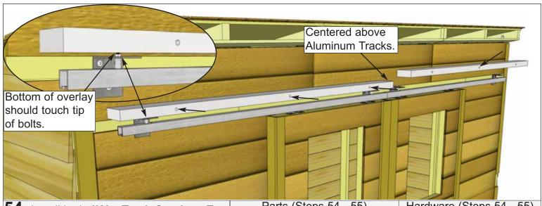
**54.** Install both **4KA - Track Overlay - Top** pieces above the aluminum tracks. Position pieces horizontally as shown above. Attach with **3 - 4" Screws** per piece through the pre-drilled holes.
