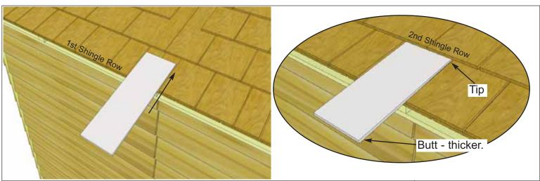
37. To cover roof seams, slide a 3I - Filler Shingle up and underneath second shingle row. Push or bang filler carefully with a hammer until evenly spaced and butt is even with other 1st row of shingles. Do first filler shingle on both seams.
