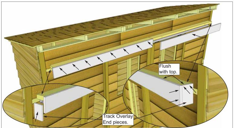
**55.** Position both of **4KB - Track Overlay - Front** onto the edge of the Overlay Top so they meet at the center. Ends of the Overlay Front will protrude 1/2" past the ends of the Overlay Top. Attach with **8 - 1 1/2" Finishing Nails** per piece.
