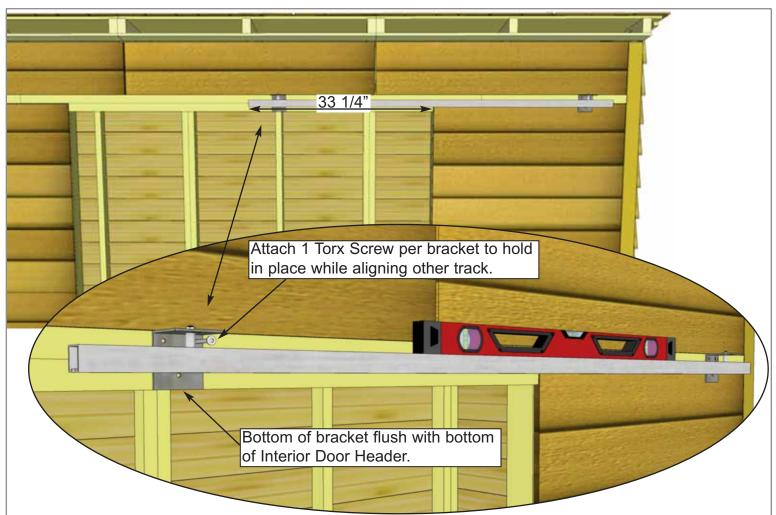
**49.** Position **4E - Aluminum Door Tracks** so they meet in the center of the doorway and with the pre-installed brackets fitting evenly on Door Headers. Ensure Track is level and attach with **1 - 1 1/2" Torx Screw** per bracket to hold in place while aligning other Track.
