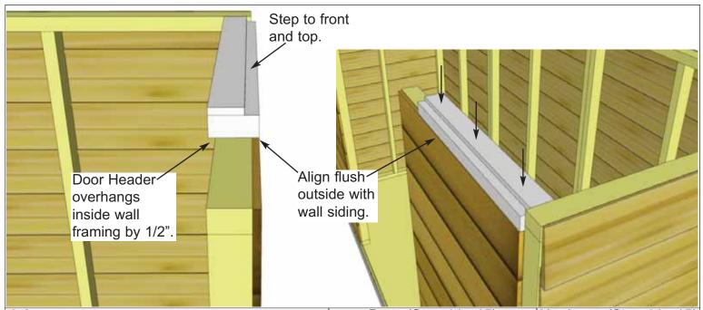
**14.** Position **2C - Door Header - Short** on top of wall stud so it is flush on the outside with the wall siding. Attach by screwing down into top wall framing with **3 - 3" Screws**.
