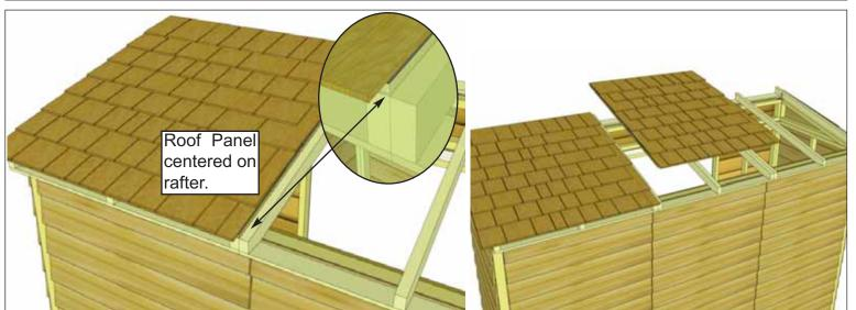
**33.** For correct Roof Panel position, align panel so plywood sits evenly on Center Rafters. Next, position **3H - Center Roof Panel** onto center rafters.
