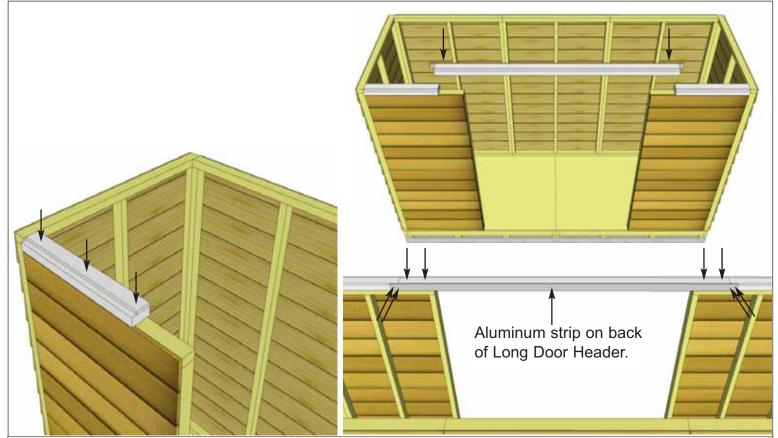
**15.** Attach **2C - Door Header - Short** to other side. Position and attach **2D - Door Header - Long** between short door headers. The Long Door Header has an aluminum strip attached to the back for added support. Attach by screwing down into wall framing with **2 - 3" Screws** per side. Fasten aluminum strip to short headers with **2 - 1 1/4" Screws** per side.
