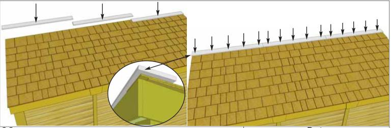
**66.** Position **4V - Roof Ridge Board** at the rear of roof to cap off shingles and facia. Ridge Boards should meet on seam of roof panels. When aligned correctly, attach with **5 - 1 1/2" Finishing Nails** per piece.
