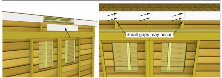
63. Attach 4T - Front Facia - Center to rafter ends as shown above. Small gaps may occur between the Center and Left/Right Facia, but these will be covered by Facia Detail Plates in Step 65. Attach with 2 - 1 1/2" Finishing Nails per rafter end.
