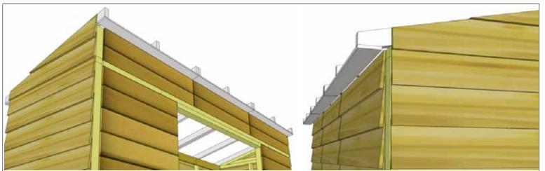
**28.** When Rafter Section is positioned correctly, both Front and Rear Soffits will sit approximately 1/8" away from wall siding. This can vary slightly.
