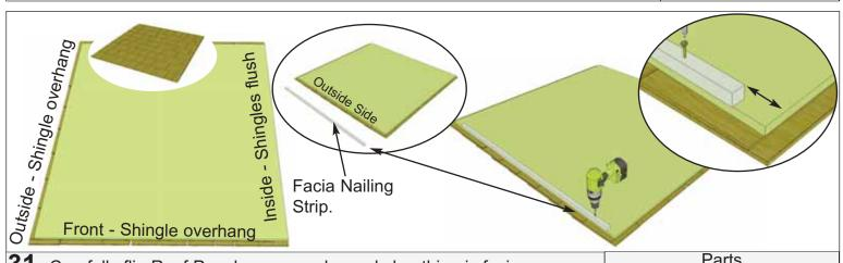
**31.** Carefully flip Roof Panels over so plywood sheathing is facing up. Center **3F - Facia Nailing Strips** onto outside of each panel flush with plywood. Attach with **4 - 1 1/4" Screws** evenly spaced. The Facia Nailing Strip provides for a greater nailing surface later when you attach side facia.
