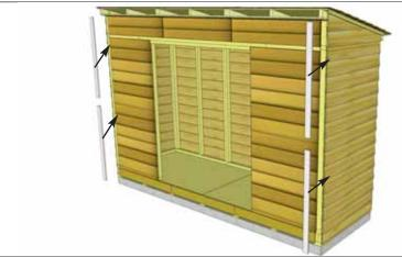
**47.** Position and attach **4C - Front Corner Filler Trim** with 4 - 1 1/2" Finishing Nails per piece. Filler trims won't be visible because they serve as nailing strips for the Corner Trims which will be attached later.
