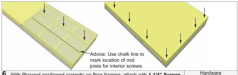
**6.** With Plywood positioned correctly on floor framing, attach with **1 1/4" Screws**. Use screws every 16" around perimeter of each floor section and 3 screws through each mid joists.
